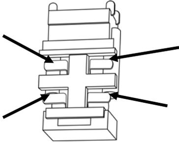
**Figure 7.3 Fuse holder with metal tabs upward**
