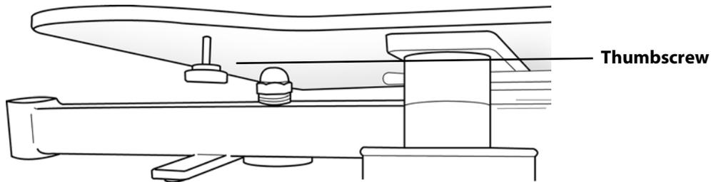
***Figure 2.1 Ventilator Base Showing Thumbscrew***
