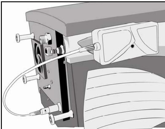
2. Attach the CO<sub>2</sub> sensor cable to the connection on the front of the CO<sub>2</sub> power box.
