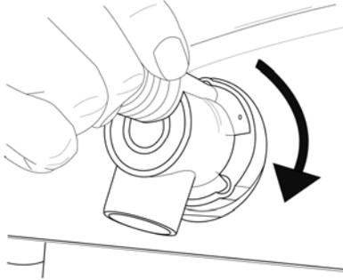
**Figure 2.4 Engaging the valve body**
