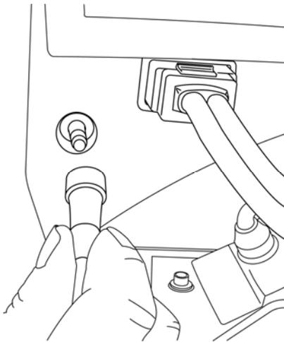
**Figure 2.8 Attaching nebulizer tubing**
