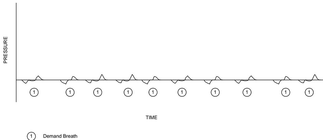
**Figure 3.11 CPAP Waveform**
