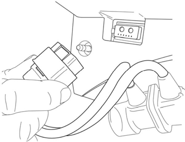
**Figure 2.6 Connecting the Variable Orifice Flow Sensor**
