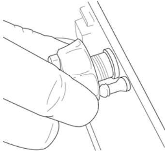
***Figure 2.10 Connecting the high pressure O<sub>2</sub> hose***
